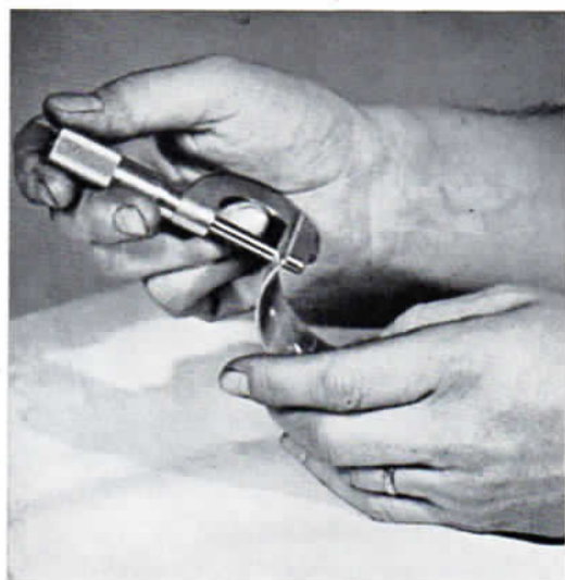
FIG. 26 CHECKING CONNECTING ROD BEARINGS WITH BALL MICROMETERS
