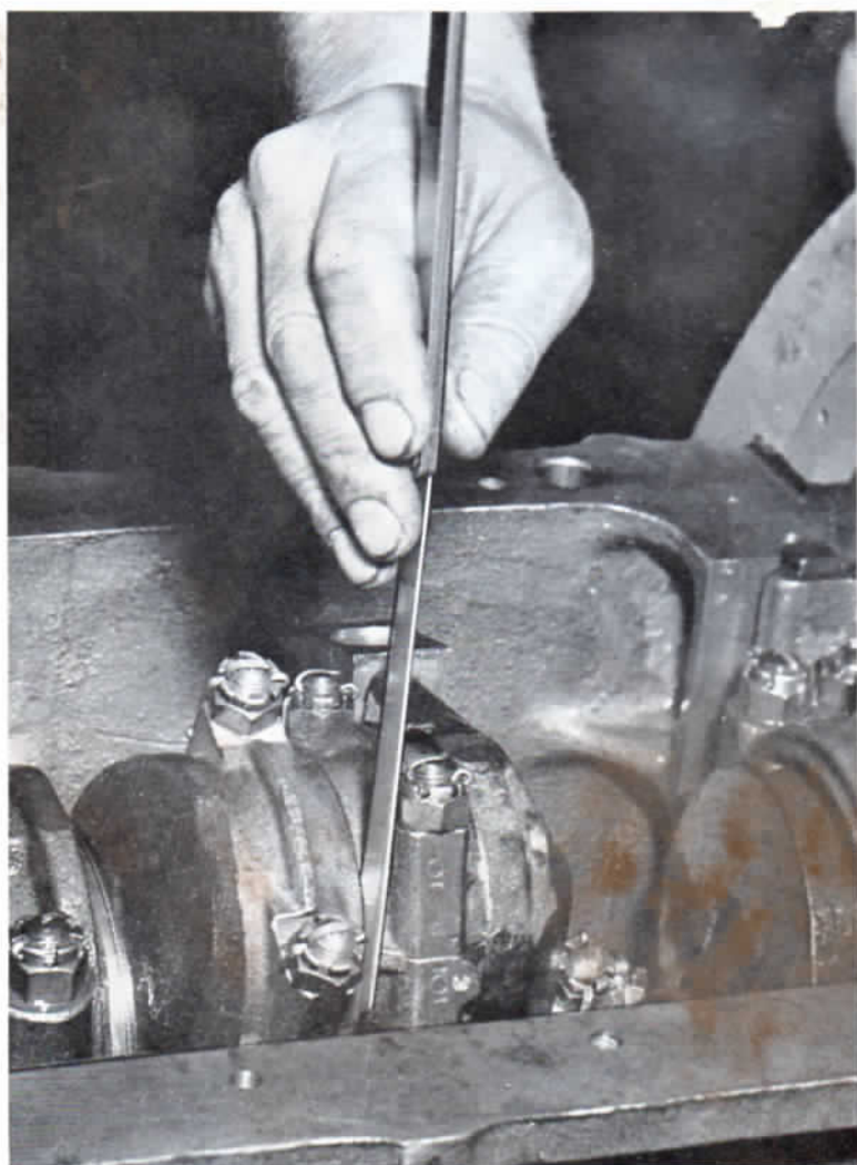
FIG. 29 CHECKING CONNECTING ROD SIDE CLEARANCE
